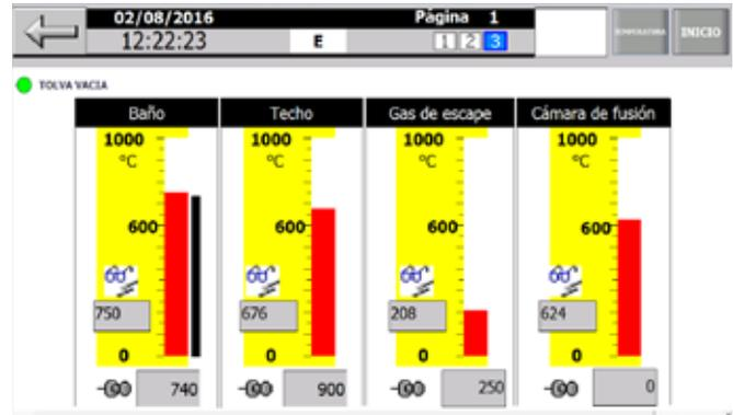
The KROWN Melting Shaft Furnaces are controlled through a control cabinet which includes a 15" touch panel from which you can obtain and control values relative to temperature, pressure or loading conditions. In addition to this, we can do monitoring of power consumption data. The software installed in the furnaces is own-engineering and includes graphics and images that make it easy to work with, and it becomes very intuitive for a better control of the melting process.
